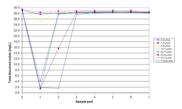
Figure 11. Diverter E's relationship between the mean total dissolved solids concentration and location of sampling ports in the diverter chamber at various flow rates with a closed diverter chamber drain.
