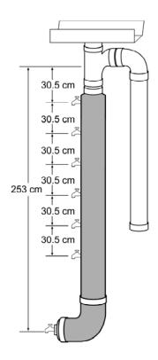
Figure 5. Diverter chamber sampling port locations relative to the diverter chamber to downspout transition fitting.
