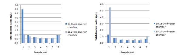
Figure 23. Comparison of the mean differences in initial and final total dissolved solids concentration in four downspout first flush diverters utilizing two downward oriented (left) and two upward oriented (right) sanitary tees at a flow rate of 3.03 L/min.
