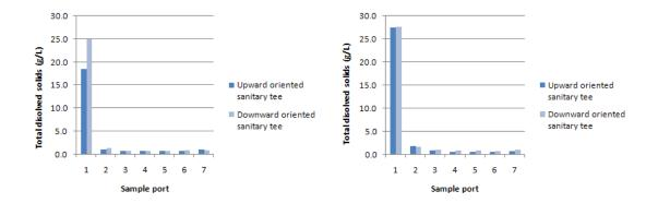
Figure 17. Comparison of the mean differences in initial and final total dissolved solids concentration in two 10.16 cm (left) and two 15.24 cm (right) diverter chambers at a flow rate of 22.71 L/min.
