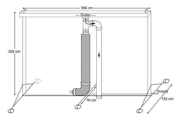
Figure 3. Downspout first flush diverter mounted on the test stand.
