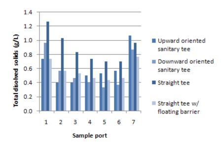
Figure 30. Comparison of the mean differences in initial and final total dissolved solids concentration in four downspout first flush diverters with a 10.16 cm diverter chamber at a flow rate of 1.51 L/min.
